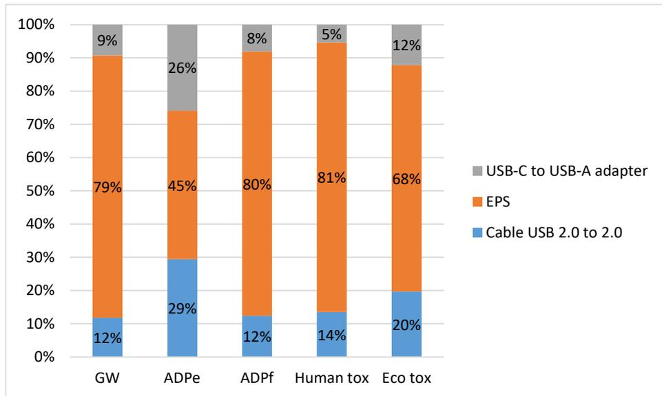
Figure 27 - Relative impacts of USB 2.0 to 2.0 charger production
