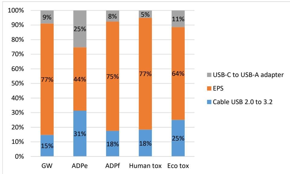
Figure 29 - Relative impacts of USB 2.0 to 3.2 charger production
