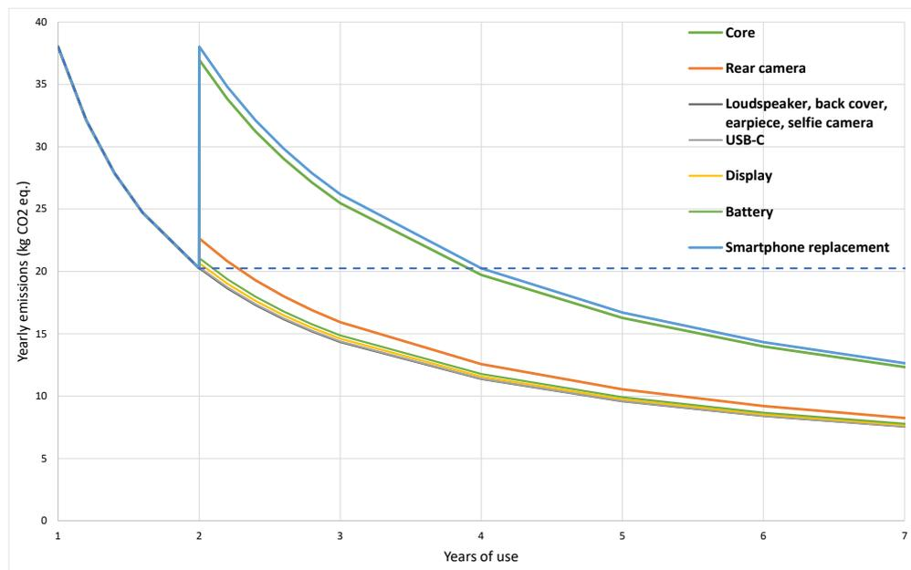
Figure 42 - Estimation of environmental payback period for module replacement, assuming failure at 2<sup>nd</sup> year of use
