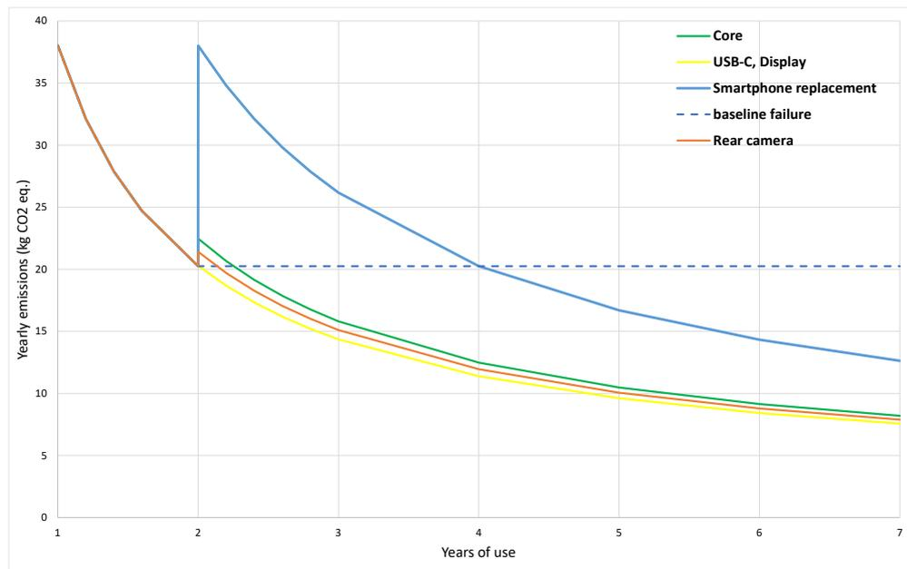
Figure 43 - Estimation of environmental payback period for module repair, assuming failure at 2<sup>nd</sup> year of use
